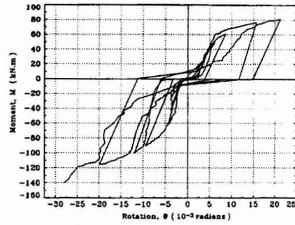
Figure 2: Hysteretic curve for non-retrofitted specimen
