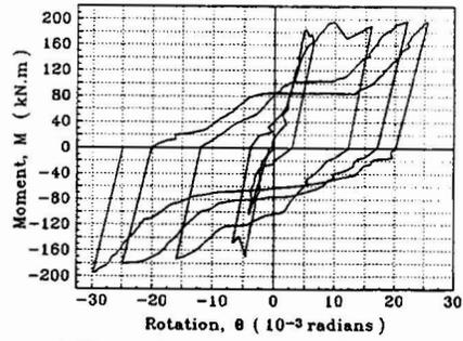
Figure 4: Hysteretic curve for tested knee braced specimen
