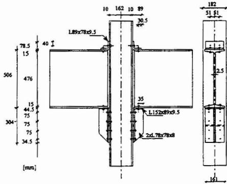
Figure 1: Detail of non-retrofitted riveted stiffened seat angle connection
