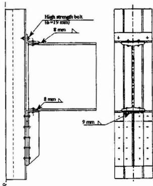
Figure 5: Specimen retrofitted using selective welding technique
