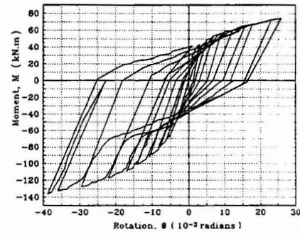
Figure 6: Hysteretic curve for tested selectively welded specimen
