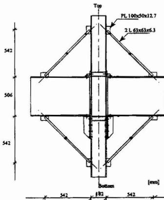
Figure 3: Specimen retrofitted using ductile knee braces
